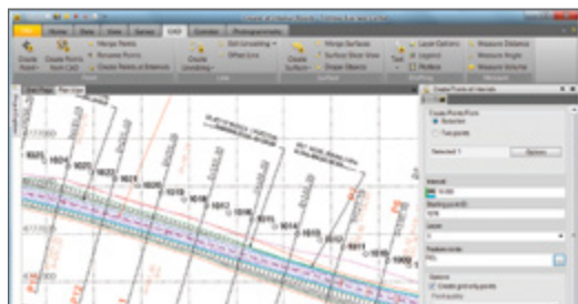
Automatically create points at horizontal and vertical offsets from an alignment for stakeout
